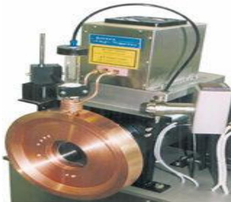
**Fig.1.** Melt-spinning Machine
