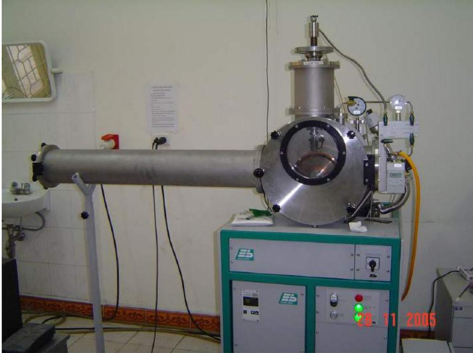
**Fig.3. Vacuum arc melting machine**
