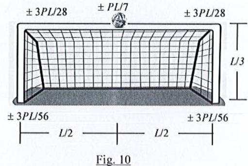
13. The goal post described in Question 11 and 12 is modified with two internal hinges at two ends of the cross bar (beam). The diameter ( $d$ ) of the cross-section is also fixed at  $d = (1 + 0.01R_0)''$ .
