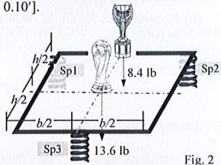
2. Fig. 2 shows the World Cup Trophy (weighing 13.6 lb) and Jules Rimet Trophy (weighing 8.4 lb) supported by three identical springs (Sp 1, 2, 3). Given  $b = h = (10 + 0.1R_0)$  ft, and the spring-deflections are not to exceed 1", determine
