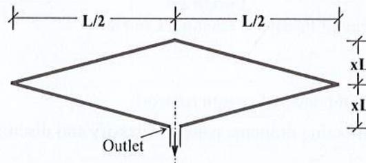
4. (a) Calculated Peak runoff ( $Q_p$ ) for the conditions of the following facility is  $2.244 \text{ ft}^3/\text{s}$ . Calculate  $L$  ( $L$  is in meter). Consider intensity of rainfall for the whole area  $1.05 \text{ in/hr}$  and coefficient of runoff for concrete, asphalt and lawn areas  $0.85$ ,  $0.75$  and  $0.20$ , respectively. 10
