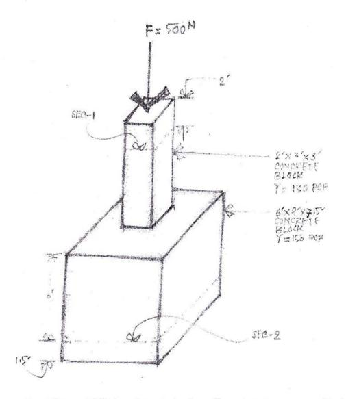
system, calculate (showing unit detail) the total stresses (due to induced load of 50 N and self-weight of concrete) in lb/in² (nsi) and N/mm² 6. (a) At sections SEC-1 and SEC-2 as shown in the above figure depicting a concrete block and self-weight of concrete) in lb/in² (psi) and N/mm².
