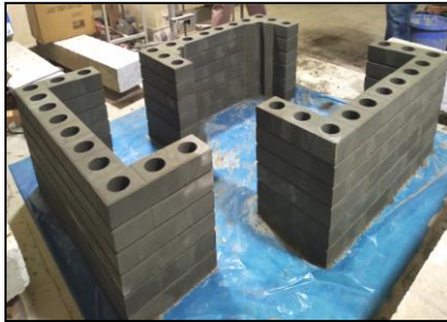
Research Walls made of Compressed Earth Block Professor Iftekhar Anam
