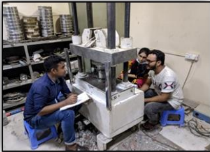
Research data collection of Compressive strength test under the project entitle “Effect of water quality on strength properties of concrete” (Dr. Mahmudul Hasan)
